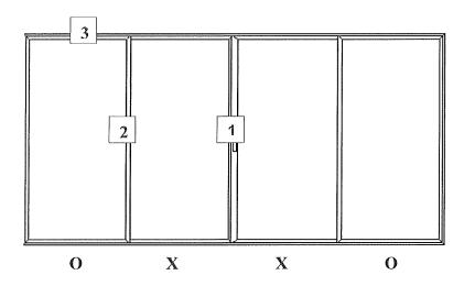
Deflection / Permanent Set were measured with three (3) dial indicators Mitutoyo control #'s A068, A067 & A070. Measurements were taken at #1 center mid-span of astragal, #2 center mid-span of interlock & #3 longest span between installation fasteners at frame head
